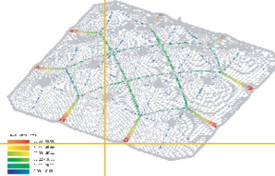
Deformation-Static Analysis Snow Load
