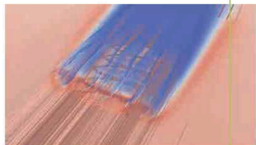
Wind Load(+X dir) By CFD Analysis
